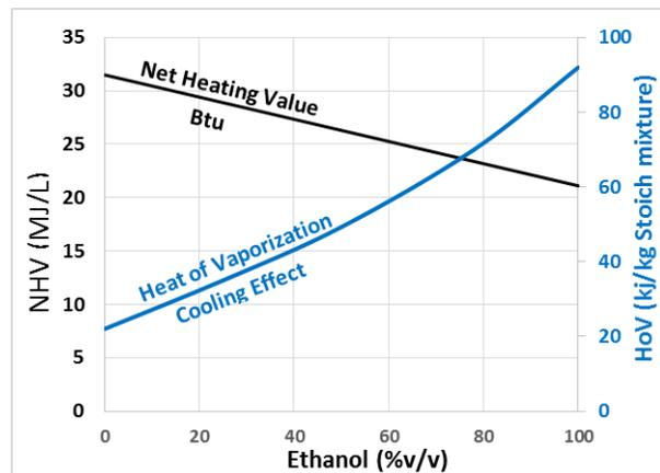
This combination of octane (RON) plus cooling effect was demonstrated in the previously mentioned [SAE paper 2012-01-1277](#), and charted in a subsequent Ford technical paper. Gasoline has a small cooling effect but, as ethanol is added to gasoline, this paper demonstrated the octane performance compared to measured octane by adding RON plus Cooling Effect. While an E30 may test at a 100 RON, the overall performance could be as high as a 106 RON.
