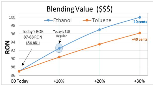
What needs to be pointed out by either the two arrows in the top chart or the RON response in the lower chart is that ethanol has nearly twice the octane increase compared to toluene if adding up to 30% by volume.
