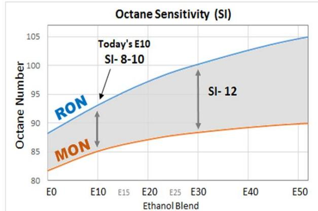
The benefit for today's engines utilizing higher sensitivity fuel enables a greater range of efficiency at higher engine load. It's difficult to raise SI at an oil refinery since most components of gasoline only offer a limited benefit. This is a huge opportunity ethanol since no other component in gasoline can compete when determining octane sensitivity.
