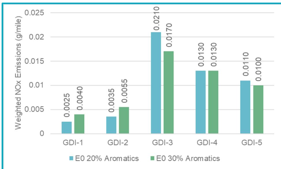
Data from Yang et al. (2019) for five GDI vehicles on two fuels using the weighted LA-92 cycle. Distance-specific emissions vary between vehicles operated on two zero ethanol fuels with different aromatic levels.
